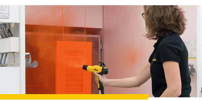
Even more efficient coating: With its innovative functions, the new Sprint 2 manual system offers a wide range of options for excellent manual coating results.
